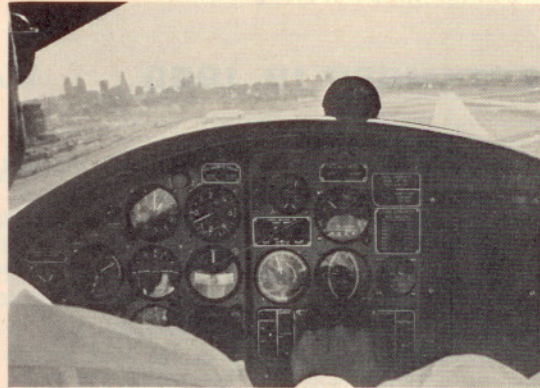
MS-760's instrument panel on final at Kansas City Municipal Airport—altitude 1,000 feet; descent, 500 f.p.m.; indicated airspeed 110 knots; engines turning 19,000 r.p.m. Note Speed Control System dial above instrument panel, showing approach to be slightly on fast side
