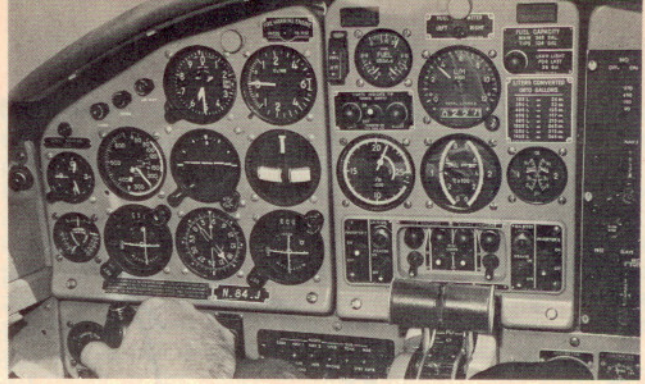
Instrument panel of Paris, shot by Jim Yarnell while the jet was cruising at 15,500 feet; Karant's hand is at the left. Airspeed indicator shows 240 knots indicated or 350 knots true airspeed; engines are turning at 21,250 r.p.m., fuel flow is about 700 liters per hour (184 g.p.h.). Photo was taken between Beech plant and Emporia, Kan., omni
